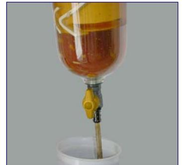
**Step 1** Turn the engine off (or switch to spare filter in duplex set up) Shut off the fuel supply valve.
