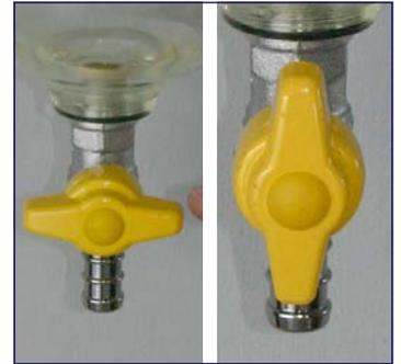
**Step 5** Drain out the water/dirt that has accumulated in the bottom of the bowl.
