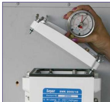
**Step 7** Fit lid checking for correct positioning. Fit lid checking for correct positioning. Evenly tighten in the sequence shown.
