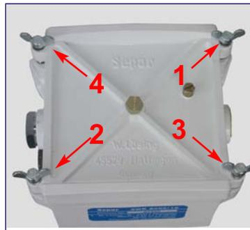
**Step 6** Inspect lid gasket. Replace if necessary.
